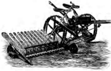
Loose sheaves grain reaper with hand operated reel
