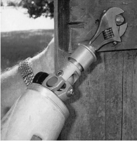
FIGURE 7.2. Modified hand tool for upper limb prosthetic user. Photo courtesy of Texas Assistive Devices, LLC, Brazoria, Texas.
