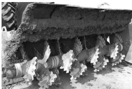
FIGURE 16.2 Tractor-mounted compost windrow turner. (Photo courtesy of Ron Wiederholt, NDSU.)
