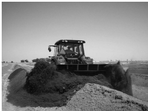
FIGURE 16.3 Manure windrow turned with mechanical compost turner. (Photo courtesy of Brown Bear Corp., Corning, IA.)
