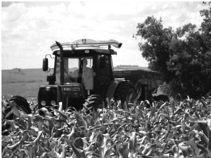
FIGURE 3.16 N-Sensor ALS (YARA) with Hércules 7.000 spreader (STARA) during top-dress variable-rate N fertilization in real time. Cruz Alta, RS. (Photo courtesy of Telmo Amado, 2009.)
