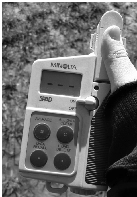
FIGURE 20.3 Image of the Minolta SPAD 502CM. (Courtesy of Konica Minolta Sensing, Inc. Tokyo, Japan.)
