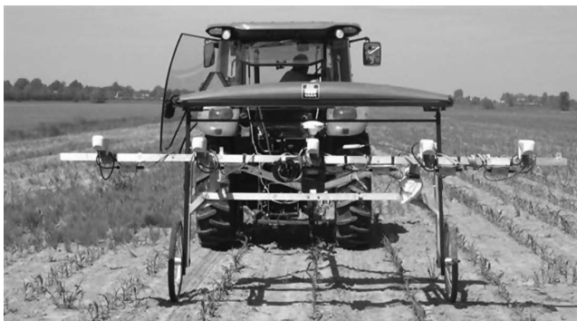
FIGURE 6.3 GreenSeeker™ sensors mounted on a trailer and pulled by a tractor designed for NDVI measurement early in the season. The setup was designed to operate over five corn rows simultaneously.
