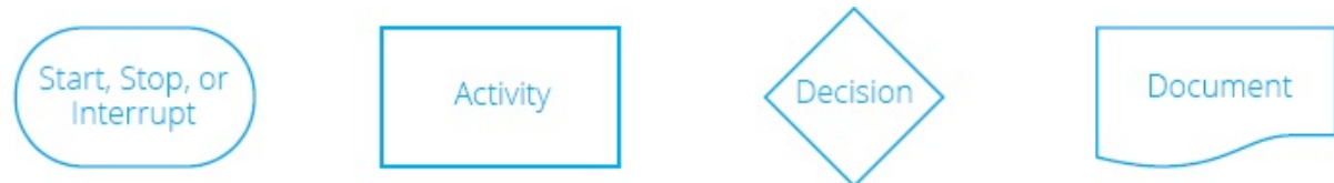
Figure 5-10. Common Process Diagram Symbols
