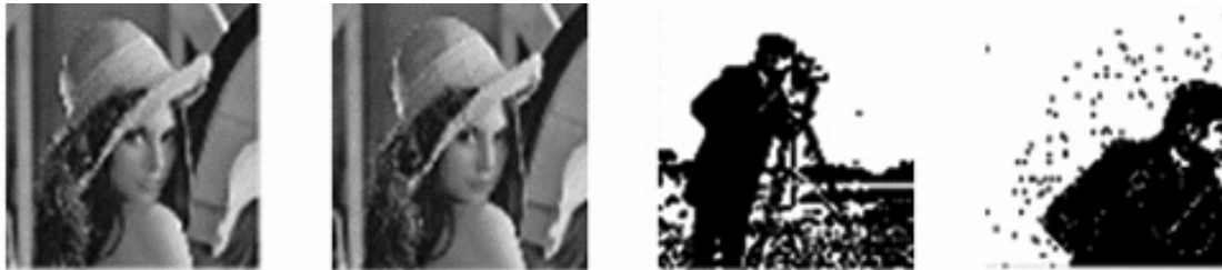
(a) Original image (b) Image after embedding (c) Watermark image (d) Watermark to extract
