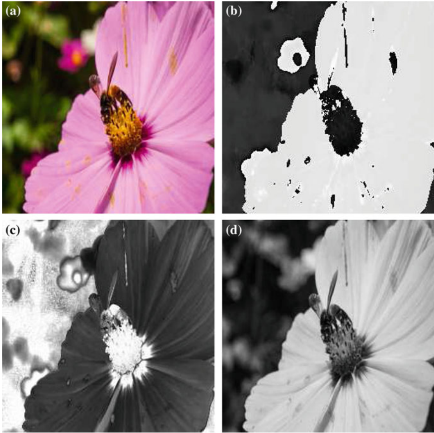
Fig. 14.9 a A 256 \times 256 color image; b–d the intensity images of the its HSI components, H, S and I in that order
