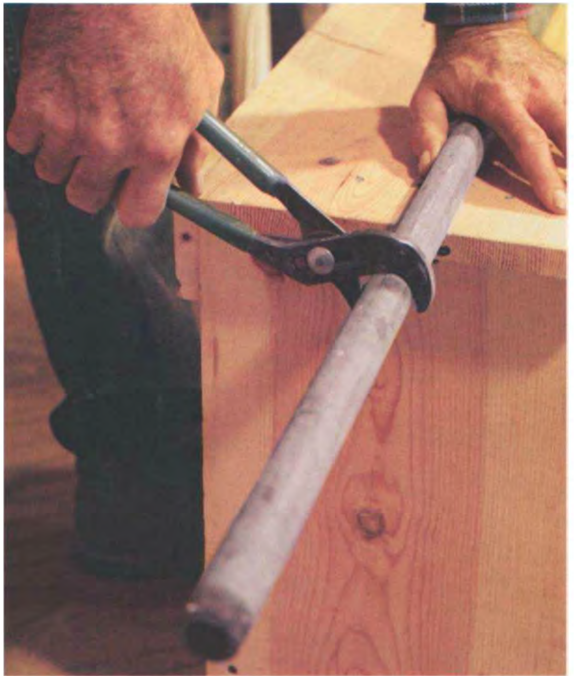
Channel-lock pliers can be adjusted like a wrench to grip pipes and other large objects.
