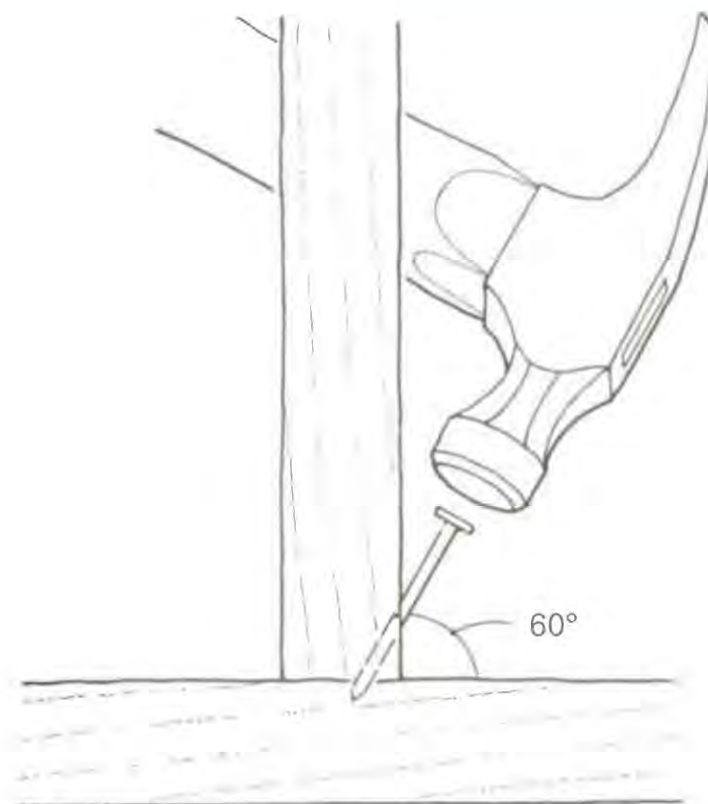
Start the nail at a 60° angle, about \frac{3}{4} in. from the end of the board.
