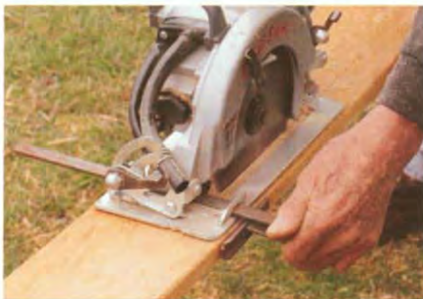
A ripping-guide attachment makes it easy to cut on a straight line, even on long stock. (Photo by Roe A. Osborn.)
