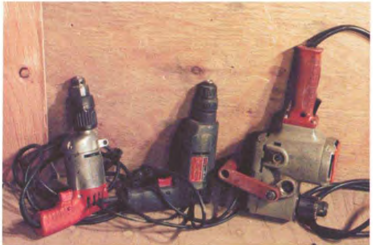
Every carpenter owns a power drill or two. Shown here are (from left to right) two \frac{3}{8} -in. pistol-grip drills and a \frac{1}{2} -in. right-angle drill.
