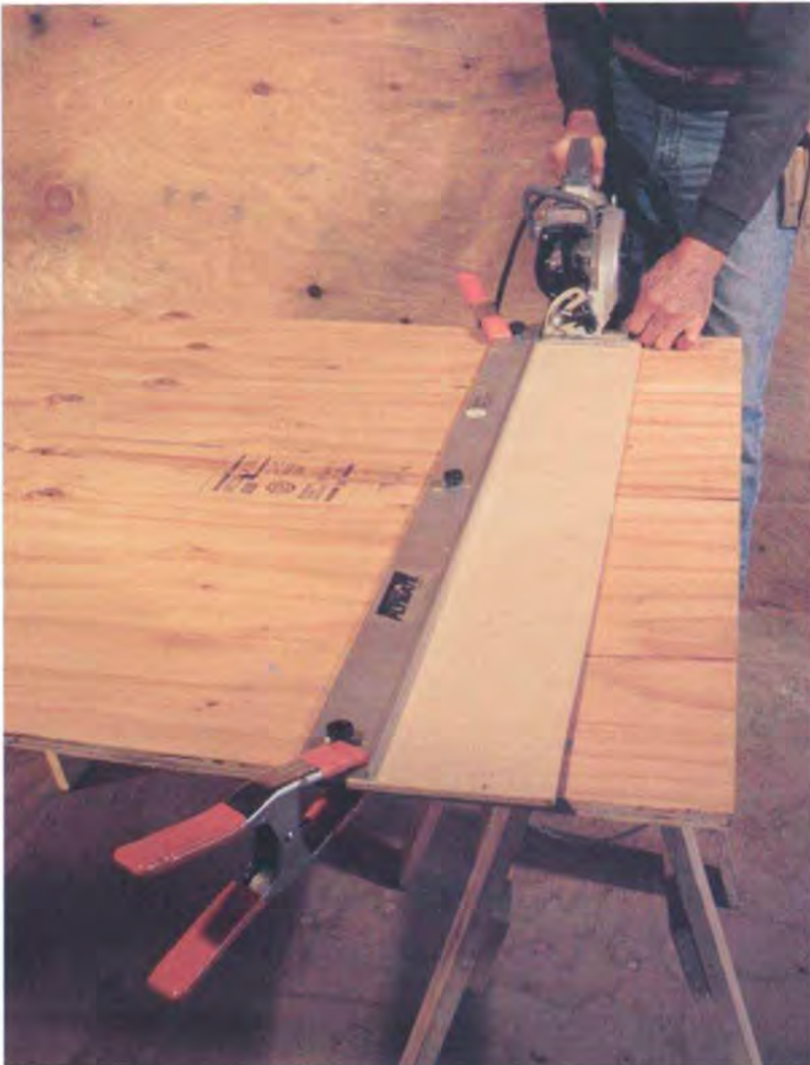
Spring clamps are quick and easy to use. Here they hold a straight-edge on a sheet of plywood.
