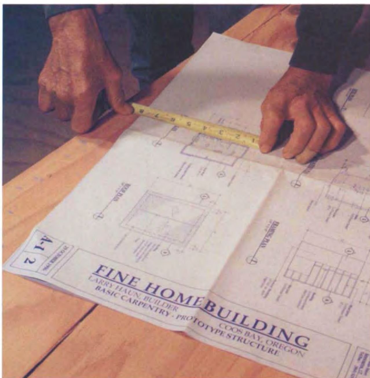
Carpenters use plans to figure out how the parts of a building will go together and to order all of the building materials.
