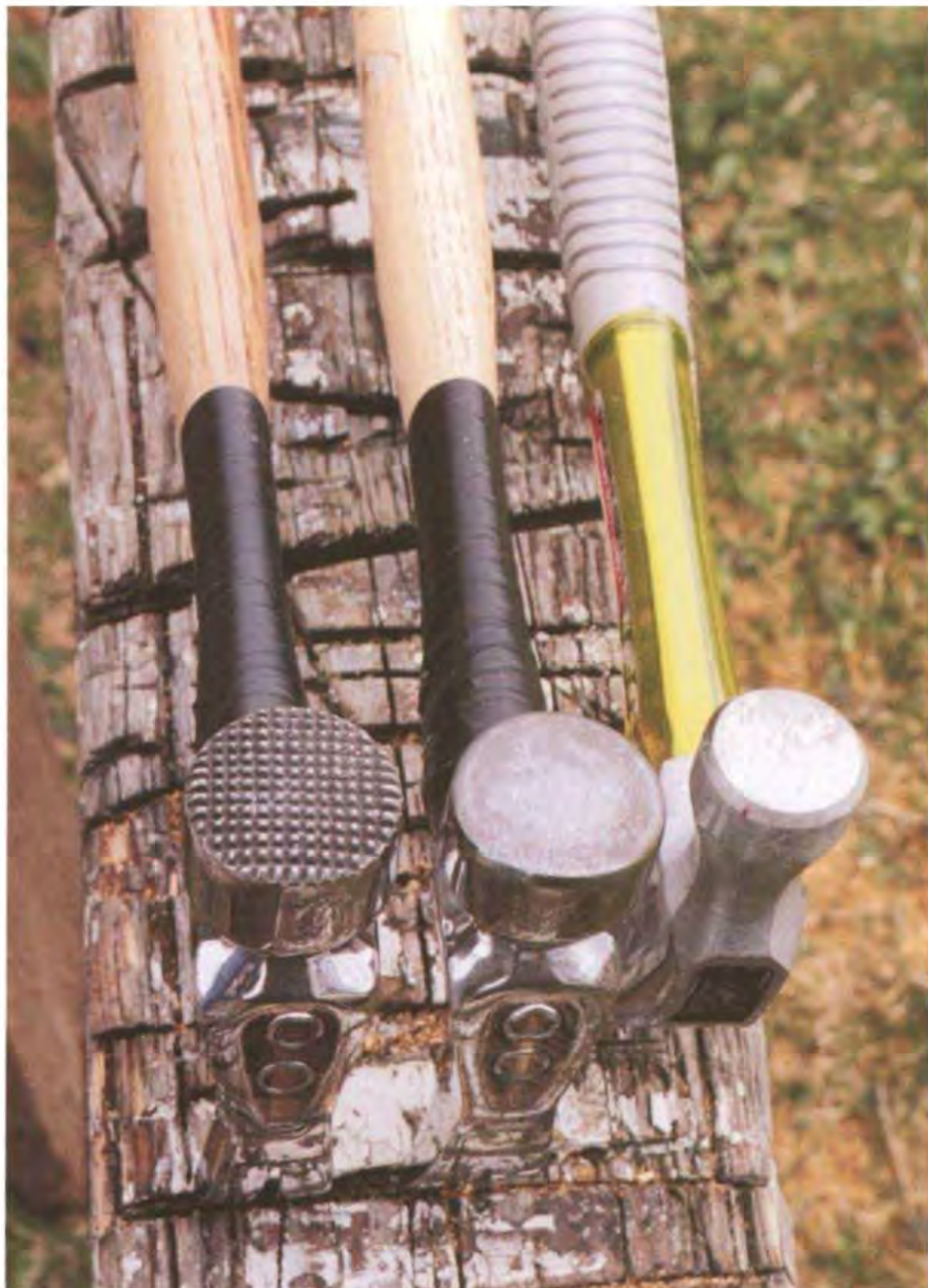
The hammer on the right has a smooth face for finish work, while the middle hammer has a face with a sandpaper texture. The serrated face of the hammer on the left grips the nail head more aggressively for tasks such as framing.
