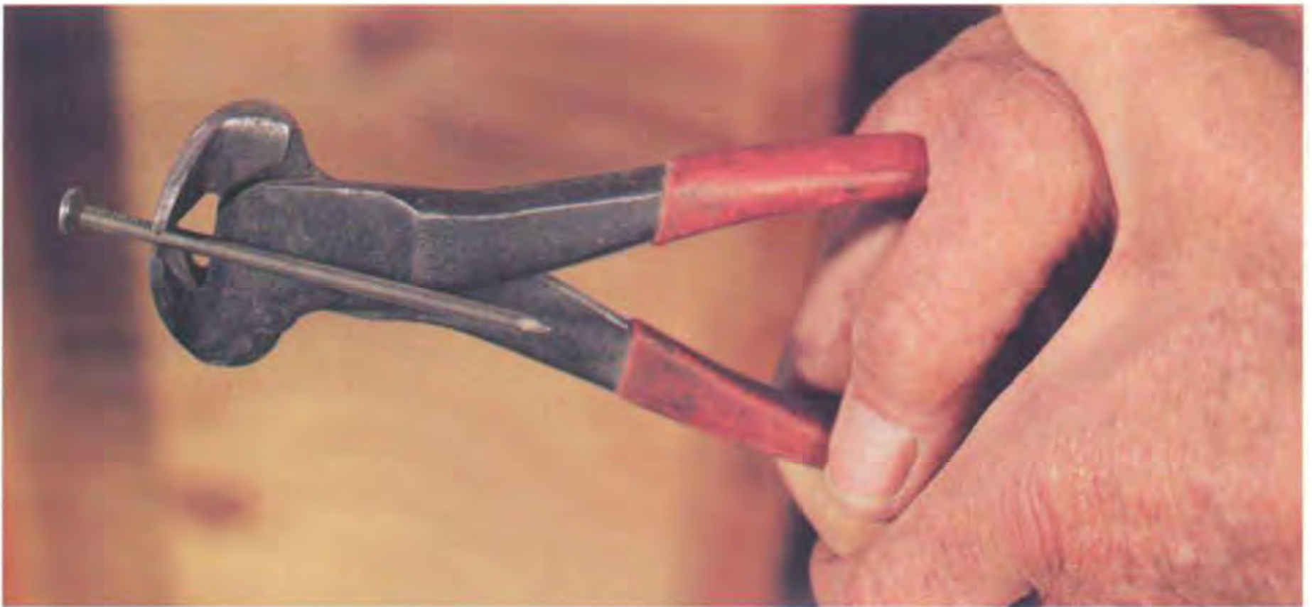
Nippers are great for cutting wire and rope and also work for pulling and cutting nails.
