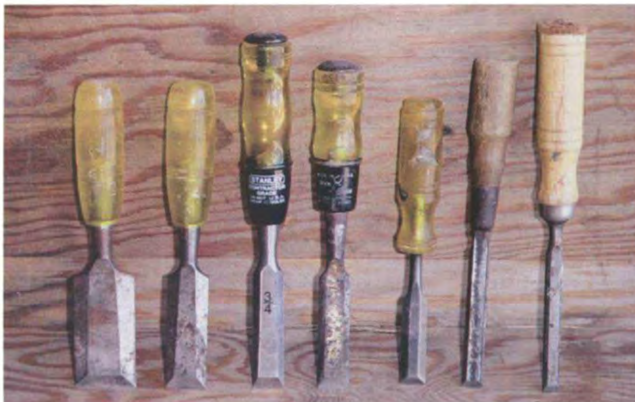
Chisels are used to cut notches in wood or to shave wood off a joint to make a perfect fit. A standard set can have sizes ranging from \frac{1}{4} in. (right) to 1\frac{1}{2} in. (left).
