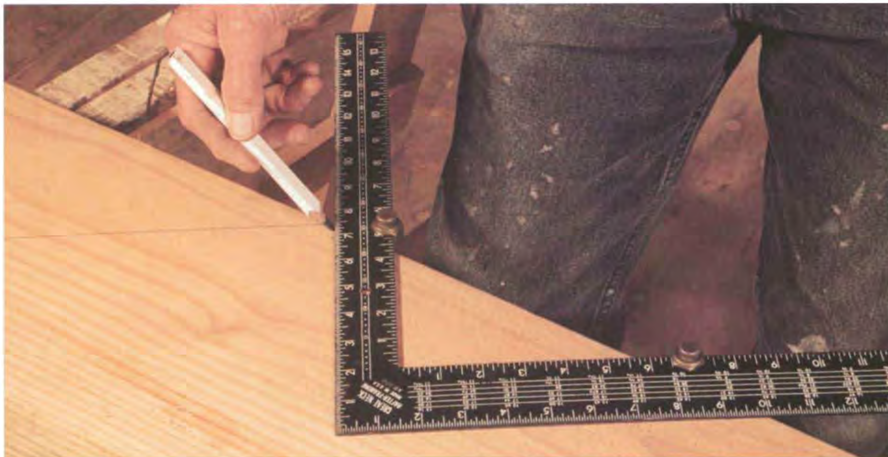
Stair gauges attach to a framing square and position it at any given angle.
