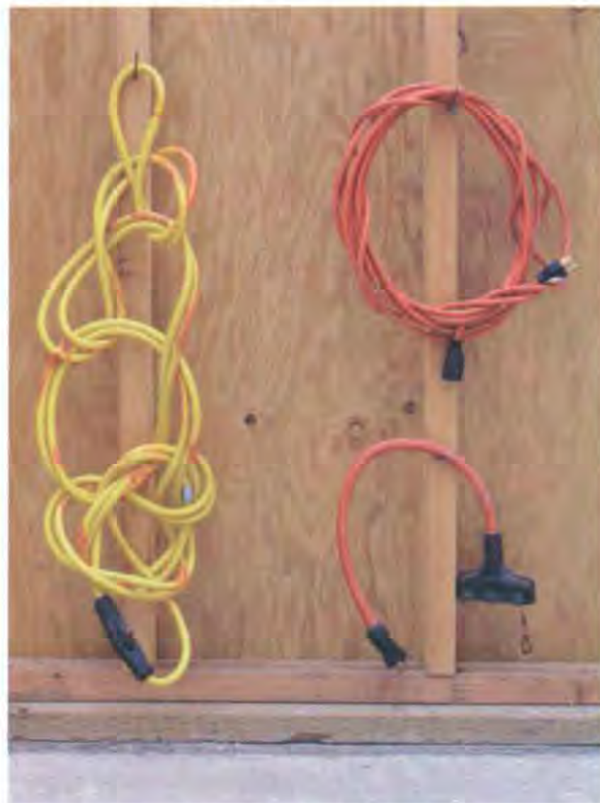
Hang extension cords from hooks when not in use. To help ensure tangle-free cords, loop them into a circle (right) or a daisy-chain (left).
