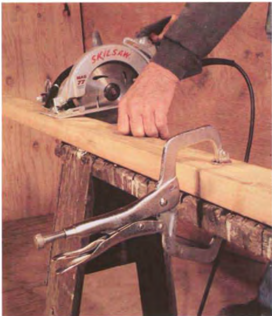
Wide-jaw locking pliers can be used to secure wood to a bench or sawhorse.
