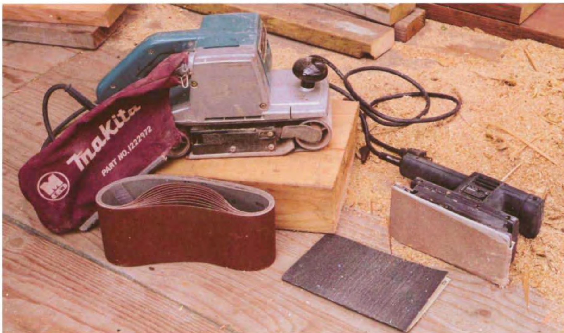
The belt sander (left) can remove a lot of stock quickly. The pad sander (right) is more suited to finish work.
