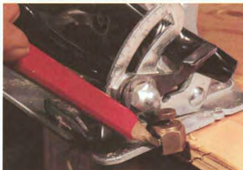
A stair gauge attached to a saw base makes a simple but effective ripping guide.
