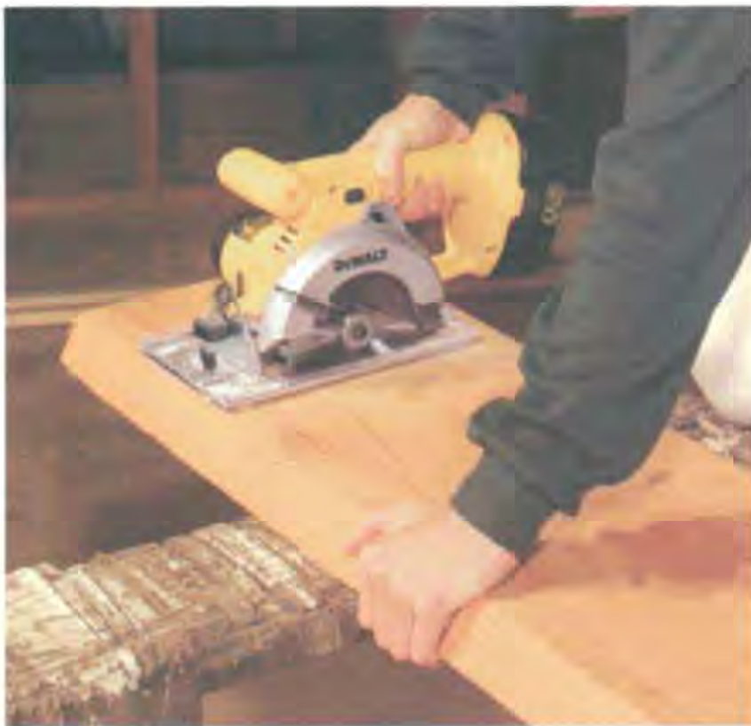
An 18-volt cordless circular saw can make short work of 2x stock.
