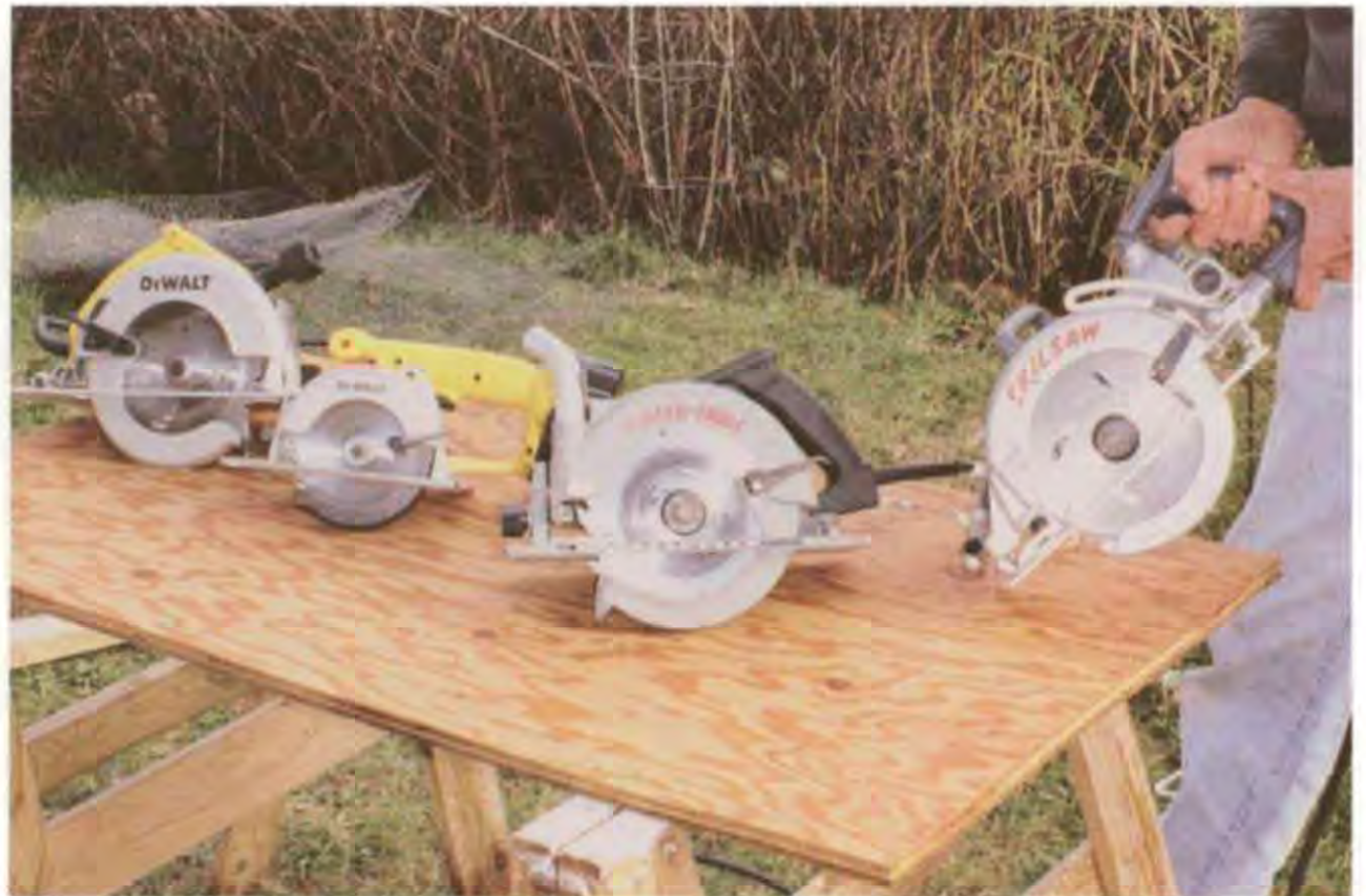
The circular saw is the workhorse of the building industry. Shown here are (from left) a 7¼-in. direct-drive sidewinder, a 5⅜-in. cordless trim saw, a 7¼-in. direct drive, and a 7¼-in. worm drive. (Photo by Joe Haun.)
