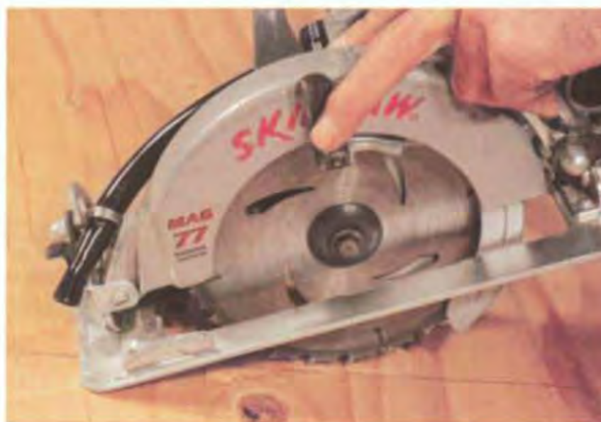
To start a plunge cut, lean the front edge of the saw base over the cut line, and start the saw with the blade about 1 in. from the wood.
