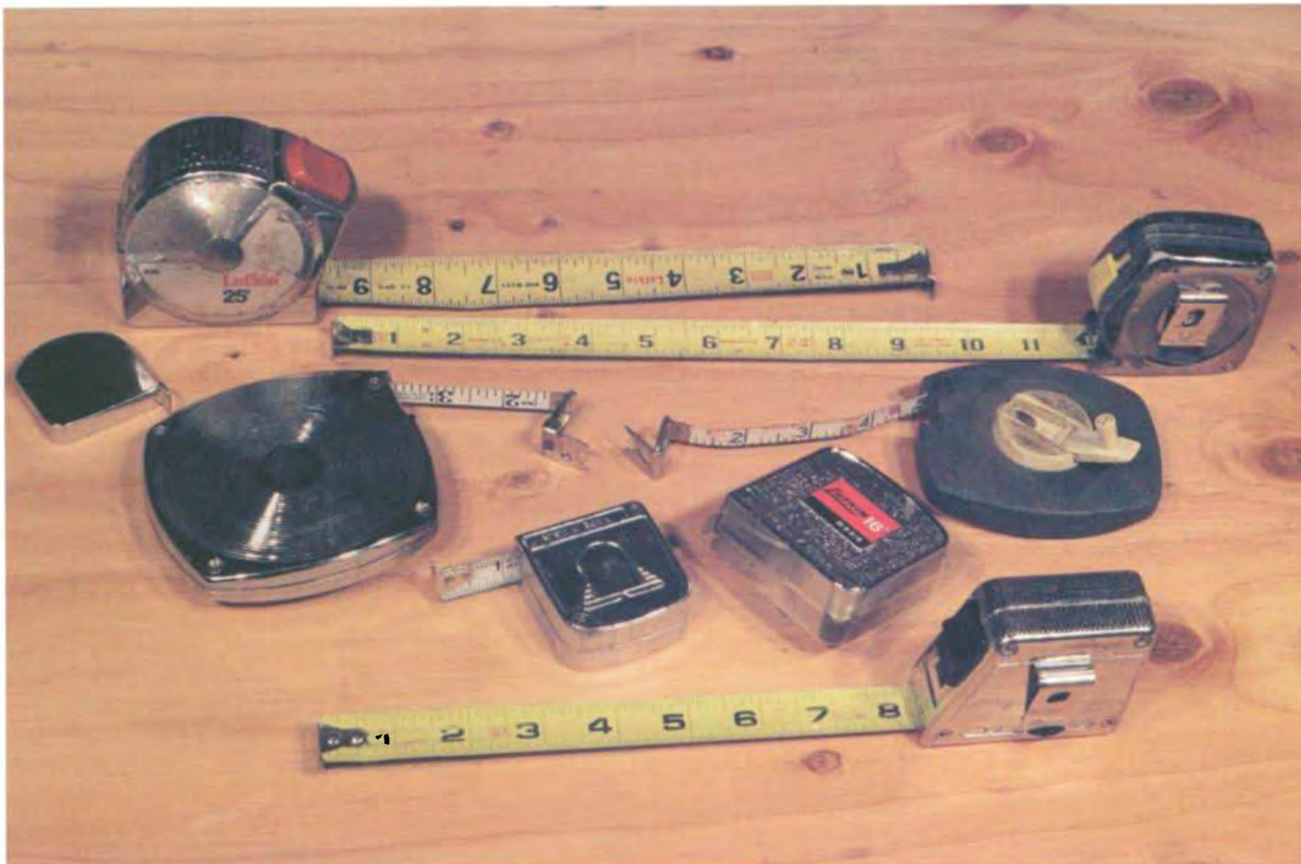
Tape measures are available in a wide variety of sizes. Most carpenters use either a 16-ft. or 25-ft. tape.
