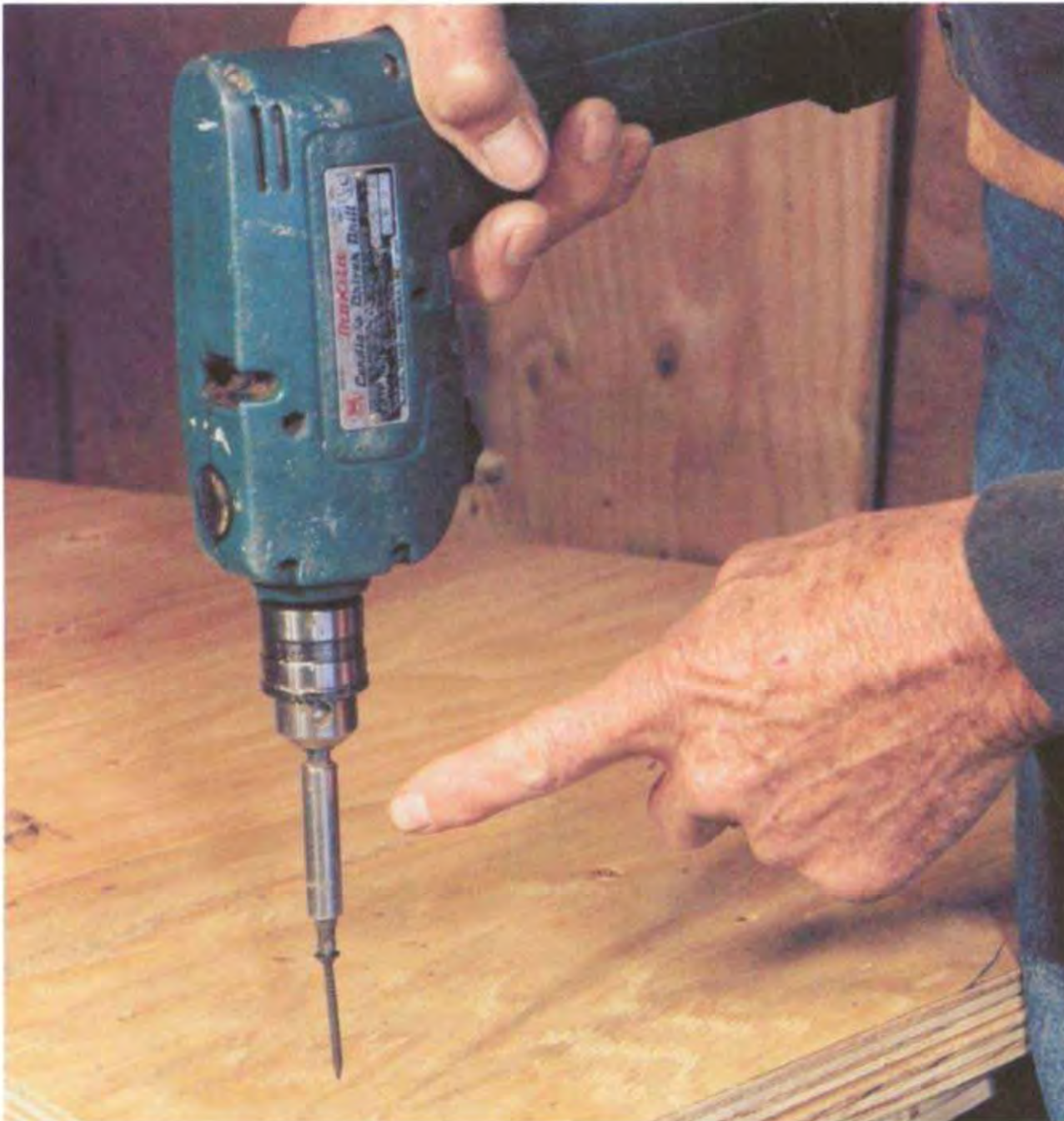
A magnetic bit holder that fits into the chuck allows you to drive screws with one hand and hold the material with the other.
