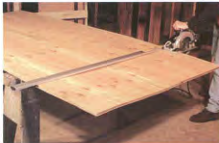
A straightedge ensures a straight crosscut.
