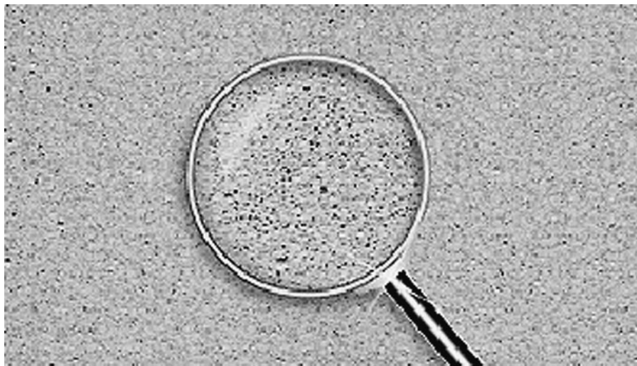
FIGURE 14.1 Close-up view of AAC.
