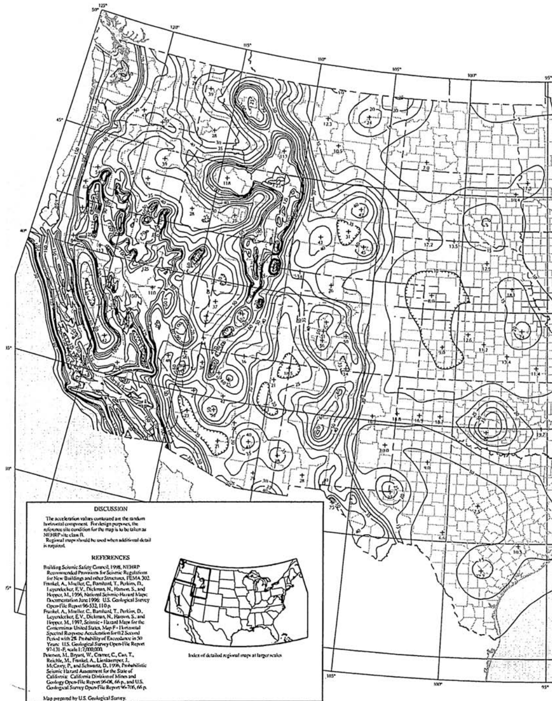
FIGURE 4.5 Contours on map of the United States showing maximum considered earthquake ground motion of 0.2-s spectral response acceleration (5% of critical damping), Site Class B. (Source: Minimum Design Loads for Buildings and Other Structures, SEI/ASCE 7-02, American Society of Civil Engineers, Reston, Va., with permission.)
