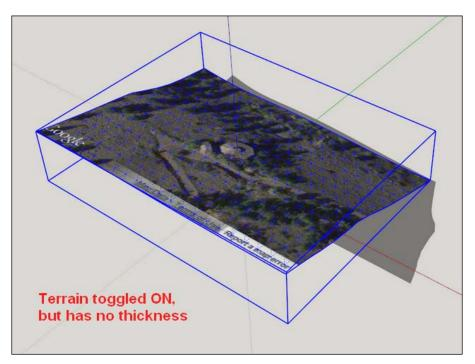
9. Now you need to add thickness to the model. This can be done manually by drawing lines down from each corner and connecting them to form a flat base. Instead, I suggest you use the extension Add Terrain Skirt (http:// sketchucation.com/forums/viewtopic.php?p=359903#p359903) to complete the task in seconds. Use the Entity Info window to ensure the terrain group is Solid before continuing. The result of this step is shown in the following screenshot:
