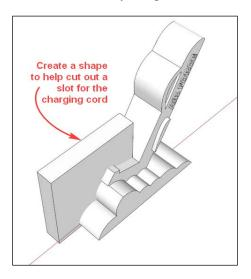
For the **Intersect with Model** command to work, the parts need to be in the same context, which means the parts to be intersected must not be in separate groups. Select the entire box and go to **Edit** | **Cut** to remove the box and copy it to the clipboard. Open the cradle group and go to **Edit** | **Paste in Place** to put all geometry in the same context, keeping the placement of the box intact.
