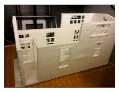
Notice how some of the windows look fine, but most of the vertical parts of the grills are missing. The tall thin posts easily get knocked over when the print head passes over them. On this second print, I added another horizontal bar across the tall windows to shorten the vertical bars. I also increased their thickness from 1.5 mm to 2 mm, but that still didn't work well. Any larger, and the grill would fill up too much of the window, so I felt cutting them out was the best option.
