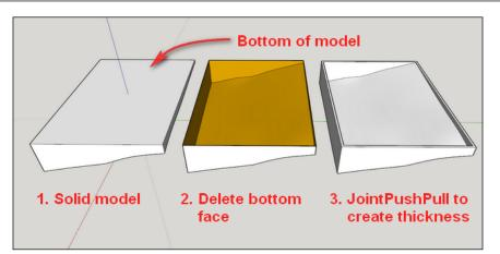
Select all, then use the right-click menu and go to **JointPushPull** | **Joint Push Pull**. Using the default options, make the terrain and walls 2 mm thick. If you encounter an error, scale the model up by 100 times and then run the operation. You may have to fix some small errors to make the model solid again. In this case, hollowing the model reduced the print material required by 85 percent.
