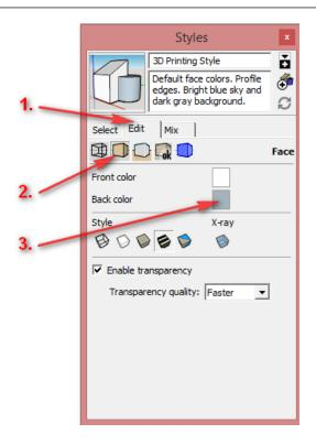
In the window that pops up, choose a nice bright color, say, orange. What this does is make it easy to differentiate front and back faces while modeling. This is important because all faces in SketchUp have a front side and a back side. The faces need to be oriented with the front faces pointing out, and all the back faces pointing inside, or the model will not print correctly.
