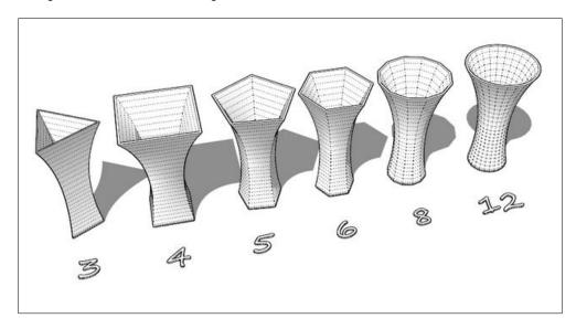
As with wall thickness, the number of segments you use in an arc should be balanced. Too many and you'll increase file size, increase processing time, and have trouble with missing tiny faces; too few and your model will look faceted and unpolished.
