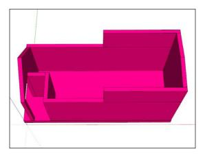
To cut the windows, turn the original model layer on and create a guideline perpendicular to the wall. Use the **Move** tool along with *CTRL* to copy and place two guidelines on each window at opposite corners. This creates two points piercing the new wall that we can use to draw a rectangle directly on the new wall and push-pull it by creating a window as shown in the following screenshot:
