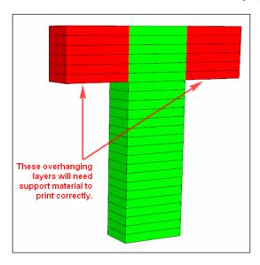
During the design phase, you should think about support material – whether it is necessary and how it can be removed. For example, printing a hollow box with a powder printer will mean designing escape holes for the uncured support powder inside; however, with FFF, escape holes aren't necessary. Often a small tweak in the design phase will make for a much better final print.
