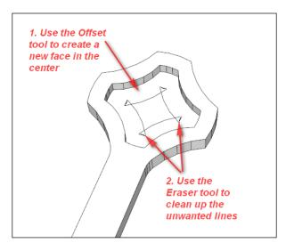
She also used the **Eraser** tool to clean up the extra lines created by the Offset operation, as shown in the following diagram. Leaving the extra lines would prevent her final model from becoming solid.
