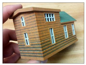
In the following image, you can see the crisp detail of the ridge seating the base of the roof to the walls. The fit is excellent, and makes the cabin look like one piece when in place:
