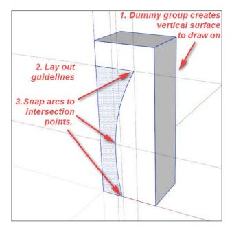
Let's break this figure down. The first thing I did was create a temporary rectangular box larger than the vase profile and make it into a group. I did this so that I had a vertical surface to draw on, making certain the profile is perfectly aligned with the red and blue axes. The box is grouped so the new geometry doesn't stick to it, and I can also use the edges of the box to assist in drawing the vertical and horizontal guidelines in the next step.
