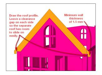
Push-pull the roof to match the length of the original model. Perform the same steps for the upper roof, and make the vertical walls to connect the space between the upper and lower roof, drawing each portion in a separate group, but combining the vertical walls and the steep roof with the **Outer Shell** tool.
