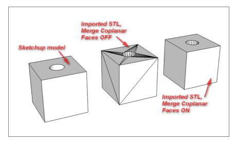
Notice the differences between the three models. The .STL format **triangulates** the model shown by the extra lines you see on the center model. The **Merge Coplanar Faces** command deletes those extra lines upon import so that you can work with imported .STL files more easily. For example, you could easily push/pull the top face of the clean imported model, but for the center model it would be much more difficult because of the extra faces.
