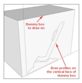
The preceding figure does not show the temporary 45 degree SketchUp guides used to ensure that the overhangs are not too steep. For more details on this technique, refer to *Chapter 4, Understanding Model Resolution*. The cloud and jet profiles are drawn as separate groups and will be joined after pulling into 3D.
