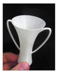
The print was a success on the very first try! Designing the handles to meet the 45-degree-overhang rule worked as intended. The printer was able to bridge the short distance connecting the top of the handle when it reached that point. The bridge could have been even smoother if I had slowed down the printer to allow cooling time for the layers below.
