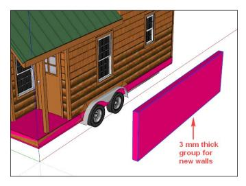
Turn off the original model layer so that it doesn't interfere, and position the new wall on the new trailer bed. Turning the original model layer on and off as needed and using the **Scale** tool just as we did with the trailer bed, align the new wall with the original as shown in the following screenshot. Scale only one direction (length or height) at a time and never along the thickness. This way the walls will all be of a uniform 3 mm thickness:
