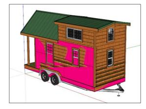
Copy the new wall to the opposite side of the cabin and repeat the process for each of the remaining walls. Notice that we *copy* the first wall to create the second, rather than drawing another from scratch. Copy and rotate the first wall by 90 degrees for the end walls.
