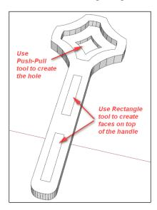
Kim noticed the opportunity to reduce material in the handle as well, so she used the **Rectangle** tool to create two faces on top of the handle, and the Push-Pull tool to create the holes. Kim was happy at this point, and exported the model as an .STL for 3D printing. The following diagram shows how the final model looks:
