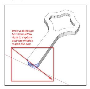
Next, Kim got the **Move** tool and moved the selected entities along the Green (Y) direction until the handle was as long as she wanted. She used the Tape Measure tool to check the length. The following diagram shows the lengthened handle:
