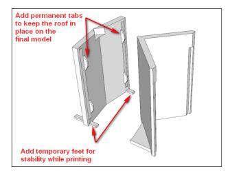
While the roofs are in the printing position, we can add more features. The shallow roof on the left has little surface area but a relatively great height. Tall, thin features like these can easily be knocked over by the print head during printing. By adding temporary feet, we can ensure that the roof will be stable for printing. These feet can be cut off with a knife after printing.
