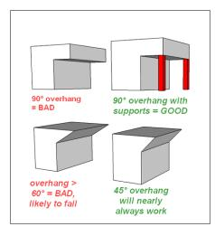
This leads to a common design rule called the "45-degree overhang rule". When designing for filament printers, keep the slope at 45 degrees or less for best results.
