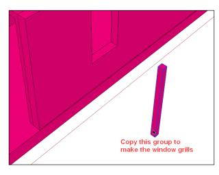
Move it into position, inferencing the midpoint of the grill group to the midpoint on the window. Scale only along the long, vertical axis as needed to fit in the window. Make a copy and rotate it 90 degrees to create the horizontal portion, and then copy these two groups to the other windows, centering them as you go. You'll want to be careful to always make sure the window grill groups are abutting or intersecting with the wall groups, leaving no gaps that will cause problems with printing.
