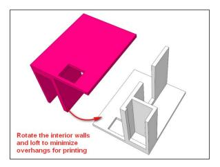
The four sections of the model can be printed all at once on the printer with no extra support, and assembled immediately afterward with little to no hand work. The only thing remaining is to combine the walls, base, and window grill groups into one solid for printing. As usual, make a copy of everything for your historical timeline before performing the operation. This way, if you need to go back and edit a particular part of the model, the separate groups make the job much easier.
