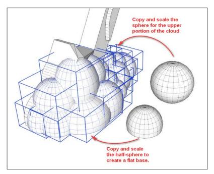
Finally, make a copy of the groups that form your new base. To prevent holes in the model when creating tiny faces in the next step, scale the model up by 100 times using the **Tape Measure** technique described in *Chapter 3, From 2D Drawing to 3D Model*. Use the **Outer Shell** tool to combine everything into one solid group. I found **Outer Shell** to work best when used on only two to three groups at a time. Selecting everything and running the tool often results in a group that s not solid.
