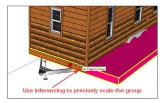
Let's make the exterior walls 3 mm thick. Create a rectangular box 3 mm wide, off to one side, as shown in the following screenshot. Make the box into a group. By copying this group and using it to create new walls in place of the existing model, we'll ensure an even 3 mm wall thickness throughout the model:
