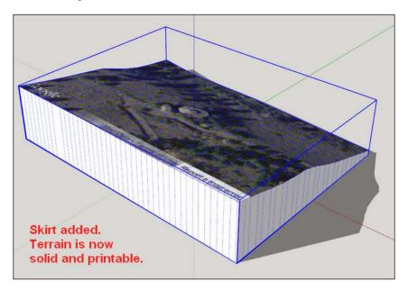
10. Since the terrain is imported at full size, the last step is to scale it down for printing. Use the **Tape Measure** tool to scale your model down using the technique we discussed in *Chapter 3, From 2D Drawing to 3D Model*. Finally, check the thickness of the skirt to ensure that it meets your preferred printer's requirements. Export the model as .stl, and you're ready to print!
