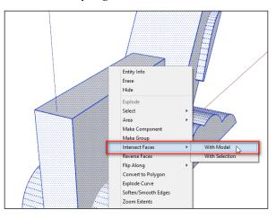
When the operation is complete, you will see that new edges have been created where the intersecting geometry meets, as shown in the next figure. Now, you can start deleting the excess geometry, taking care not to delete anything you want to keep.
