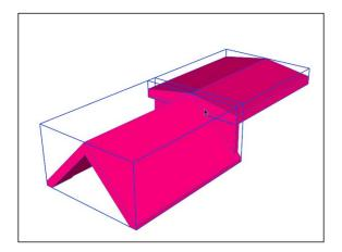
The two roof pitches are kept separate for printing on the FFF printer. Since the two roofs overlap in the center of the cabin, I used the **Subtract** tool in SketchUp Pro to cut away the portion that was overlapping. You can perform the same action using the **Intersect with Model** command in SketchUp Make. For more information on the **Intersect with Model** command, please refer to *Chapter 6, Designing a Phone Cradle.*
