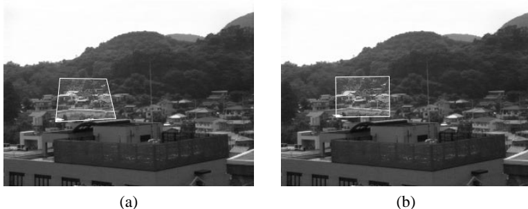
Fig. 6. (a) The image mapping computed by an optimal homography. (b) The image mapping by model selection.
