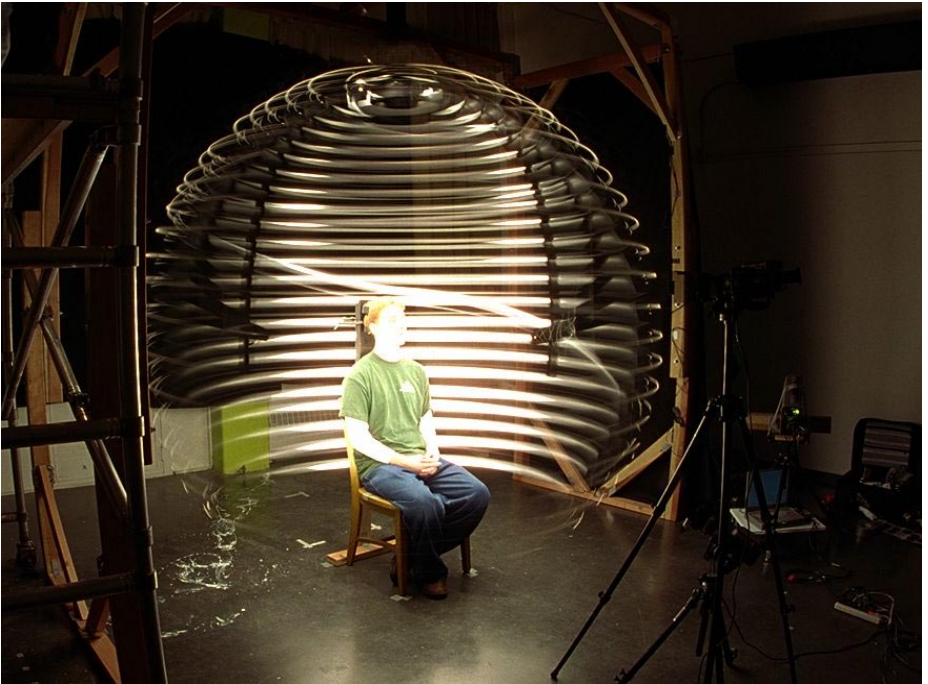
Fig. 7. Light Stage 1.0. The Light Stage [3] is designed to illuminate an object or a person’s face all possible directions in a short period of time. This allows a digital video camera to directly capture the subject’s reflectance field : how they transform incident illumination into radiant illumination. As a result, we can then synthetically illuminate the subject under any form of complex illumination directly from this captured data. Renderings of synthetically illuminated faces can be found at http://www.debevec.org/Research/LS/ .
