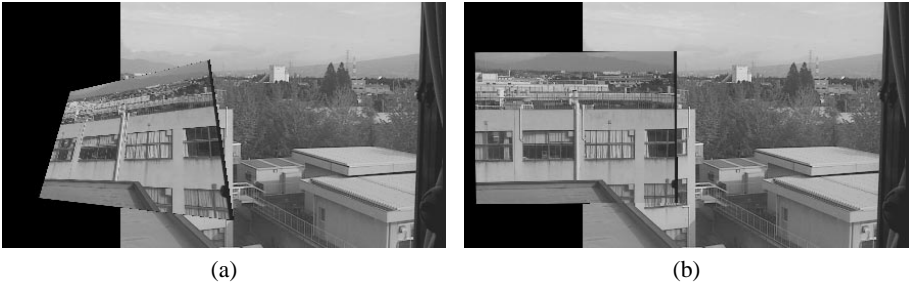
Fig. 8. (a) Mosaicing by an optimally computed homography. (b) Mosaicing by model selection.
