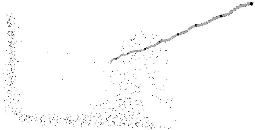
Fig. 3. The small dots on the background represent the recovered crude 3D environment. The larger dark spots represent camera positions of keyframes in the video stream. The lighter spots represent the camera positions of the remaining frames.
