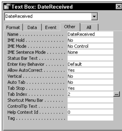
Figure 9-16: Use the TabIndex property to control the tab order of the controls on a form.
