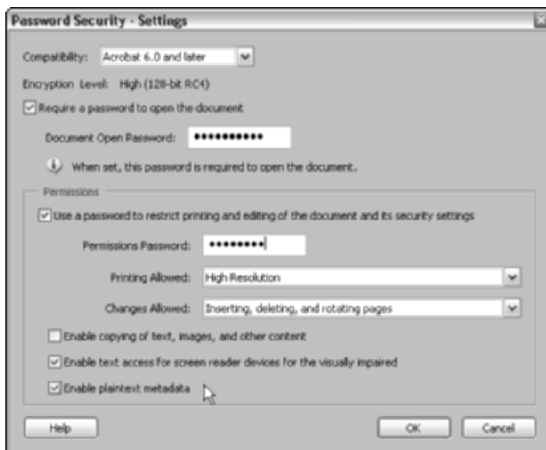
Figure 11-3: Setting the security options for 128-bit RC4 encryption in the Password Security - Settings dialog box.
