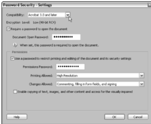
Figure 11-2: Setting the security options for 40-bit RC4 encryption in the Password Security - Settings dialog box.
