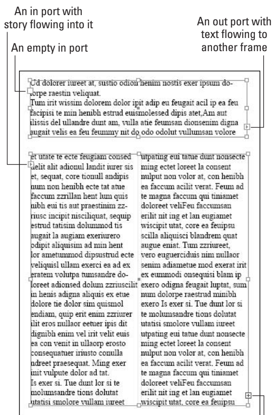
Figure 3-10: The in port and the out port depict threaded text frames. A special icon shows if text extends past the text frame and is not threaded to another frame.
