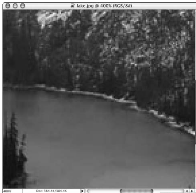
Figure 6-1: This bitmap image is made up of many pixels, which you can see when you zoom in or resize the image.
