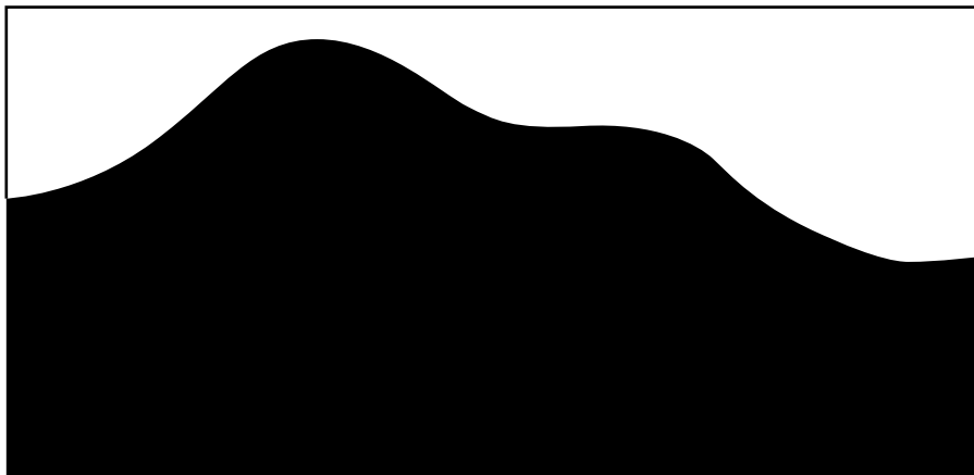
Figure 4-1: Analog data is infinitely variable.
