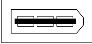
Figure 2-1: The FireWire port on your computer should look something like this.
