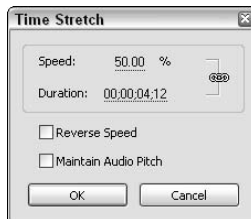
Figure 8-13: Use the Time Stretch dialog box to change a clip's playback speed.
