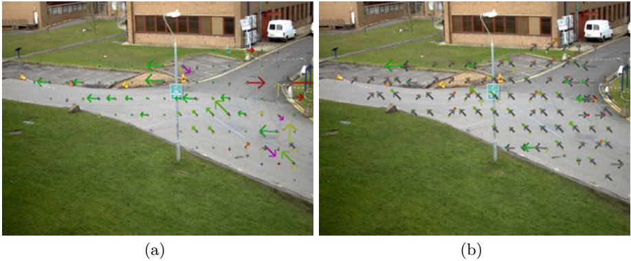
Fig. 3. Raw and regularized transition fields for an upward initial direction ( v_t^\theta = -\frac{\pi}{2} ). We depict, before and after regularization, the 3D cell having the maximal bin value, with a first arrow pointing to \mathbf{r}_{t+1} and a second arrow having orientation v_{t+1}^\theta .
