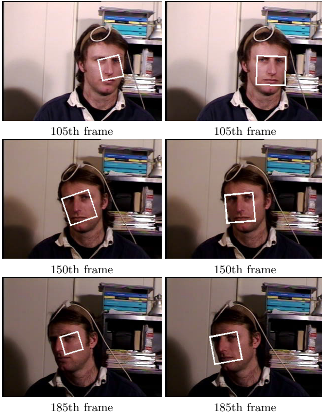
Fig. 4. Comparison of tracking jal6 (left:tracking with directional eigentemplate learned from jal3 ,right:tracking with directional eigentemplates learned from jal3+jal5 )
