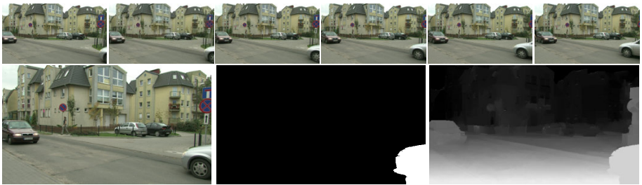
Fig. 10. The 130 th frame in the data set “Poznań”. (a) The reference frames. (b) The current frame. (c) The white region is the detected moving object. (d) Final depth map.
