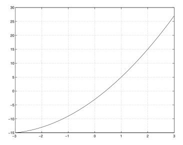
We have given the plot a grid by using the command grid on; this can be removed using the command grid off.
