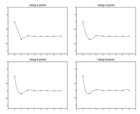
Here we note that the lower-order polynomials produce reasonable approximations; it is only when we try to fit an octic to the data we observe the problems at the right-hand end. We need to be aware the accuracy of our interpolated values is very dependent on the fidelity and resolution of the starting data.
