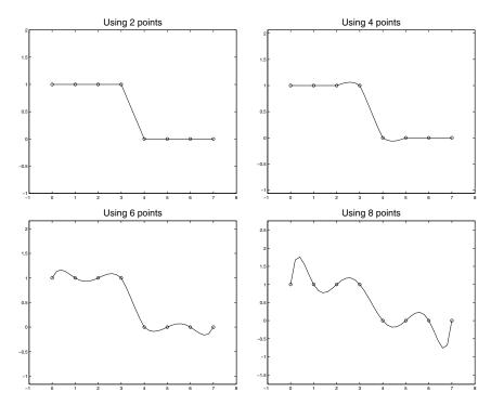
As you can see as more points are used in the interpolation, the approximation gets steadily worse and the effect extends far from the discontinuity (which is causing the problem): in fact less points seem to produce less error. The question remains as to what is the "real" data (it could actually look like the figure in the bottom right – although this is not likely).
