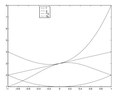
We have added a legend which uses the line styles to show which lines we have plotted. We could have used different style lines. We have used the additional argument at the end of the legend command ,0 to tell MATLAB to put the legend in the "best" position.
