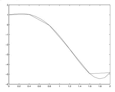
As you can see using six points works quite well at fitting the data. Although as we will see in subsequent examples using high-order polynomials can lead to significant errors.
