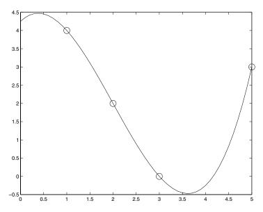
By way of illustration we shall now construct the splines through the points  $(x_1, y_1), (x_2, y_2), (x_3, y_3)$ .
