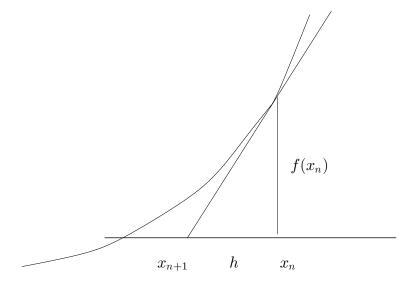
The value of h is determined by using the fact that the ratio of the two sides h and  $f(x_n)$  has to be equal to  $f'(x_n)$ .
