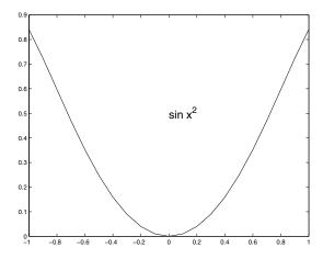
The syntax is text(a,b,string) where (a,b) is the coordinate in terms of the data and string is enclosed in single quotes. Notice here that  $\texttt{sin } \texttt{x}^2$  actually appears as  $\texttt{sin } \texttt{x}^2$ . These commands also recognise underscore for subscript and Greek letters in the form \omega, for instance.
