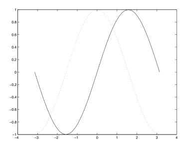
from which the command syntax can be deduced; a plot of  $\sin(x)$  versus x using a solid red line and a plot of  $\cos(x)$  versus x using a blue dotted line (if the plot were to be viewed in colour). This could have been achieved in another way
