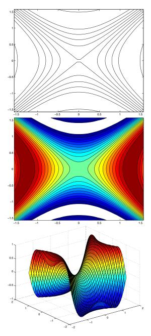
These figures are, respectively, a contour plot (created using contour(X,Y,f)), a filled contour plot with 20 contour levels (created using contourf(X,Y,f,20) and a surface plot (created using surf(X,Y,f)). The function f is plotted on a grid generated using the command meshgrid(x,y). As the name suggests
