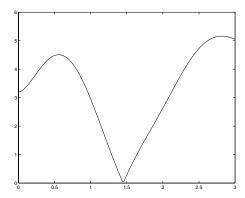
We now remark that in order to find the values of this minimum we could use search methods. But here we make the observation that one is seeking a minimum of the function, which is associated with a zero of the derivative of the function. We shall use the Newton-Raphson method modified for looking for zeros of f'(x), which is
