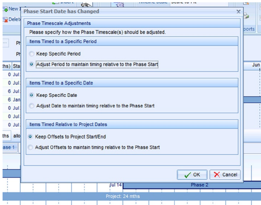
Figure 4-76. Program automatically adjusts timing but gives users the option to adjust timing as well
