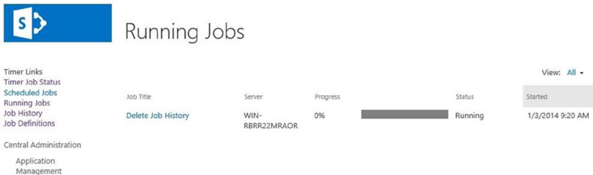
Figure 8-11. Central Administration showing the execution of a timer job triggered by PowerShell
