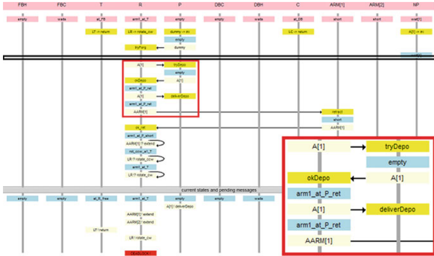
Fig. 2 The counterexample of a deadlock found in the server view of a 1-blank Production Cell
