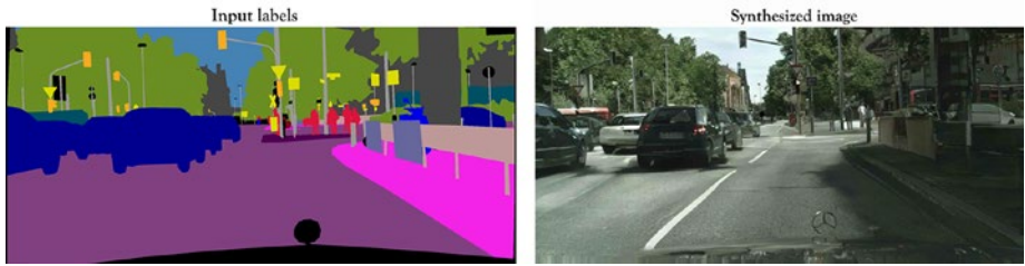
Figure 4-14. Example of high-resolution Pix2pix from Nvidia team. Left: the segmentation map; right: one possible high quality generated image (source: https://github.com/NVIDIA/pix2pixHD ).
