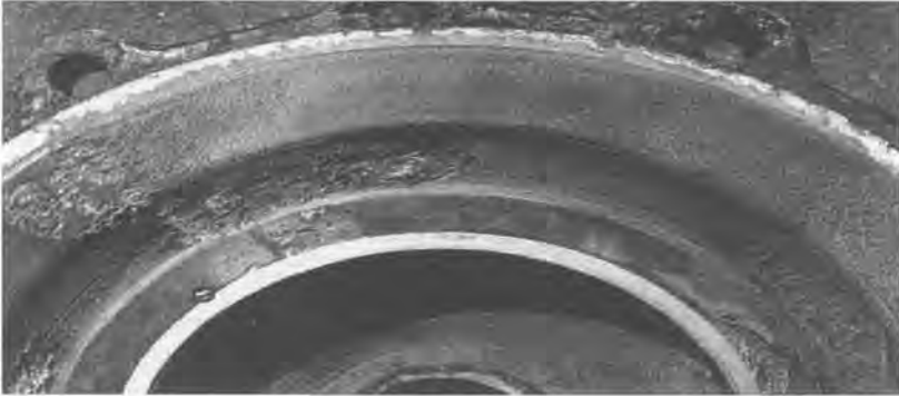
Figure 7.28 Corrosion occurred at weld repair portion of aluminum bronze casing
