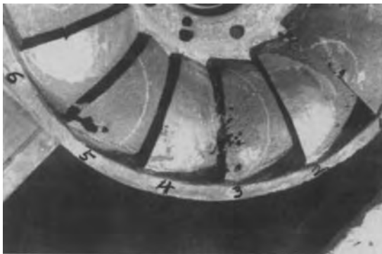
Figure 5.30 Comparison of spraying and non-spraying blades after 15,840 hours operation in Ba Jia Zui Power Plant
