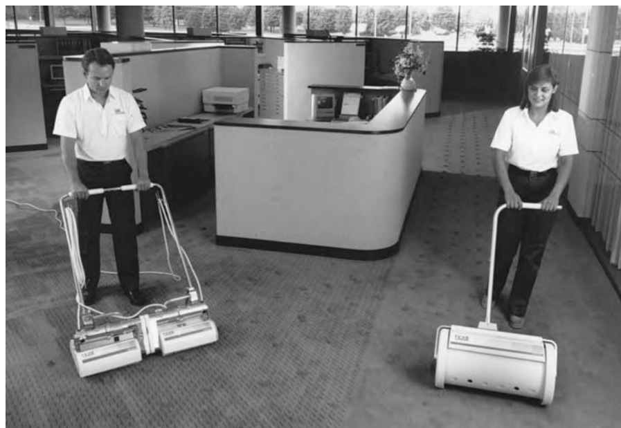
Figure 5-16 The Host Dry Powder System. The powder applicator is on the right; the dry cleaning machine on the left brushes the powder into the carpet. (Used with permission of Racine Industries.)
