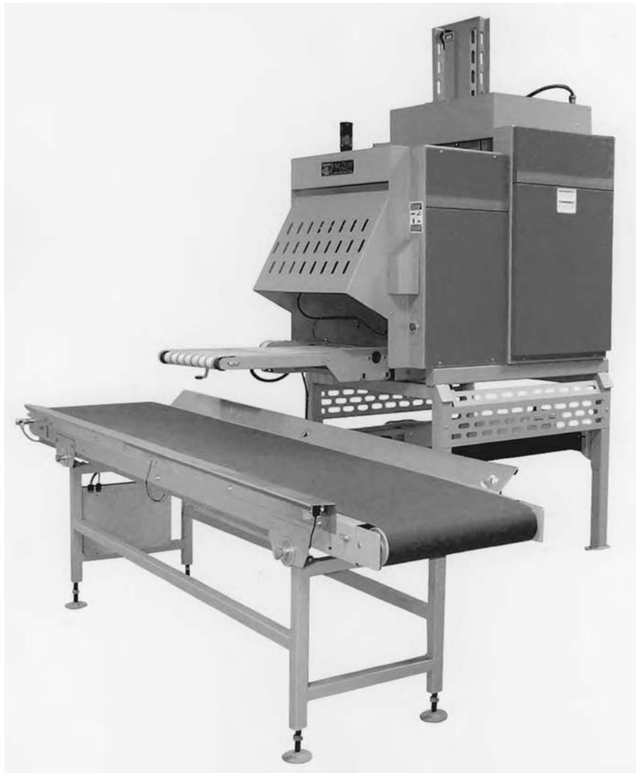
Figure 15-31 The Pik-Quik can be teamed with the Linen Stream, ™ a conveyor system that advances linen to operators who are loading a spreader/feeder like the King Edge. (Photo courtesy of Chicago Dryer Company.)
