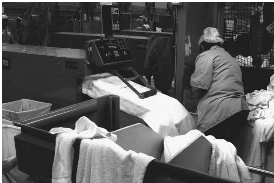
Figure 15-8 A worker feeds a towel into a folder. (Photograph courtesy of Mission Industries, Las Vegas.)
