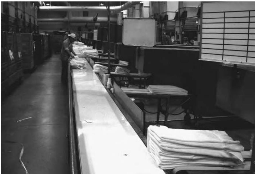
Figure 15-10 The towels proceed down a conveyor, where a worker ties them into bundles and they are stacked back into waiting carts. (Photograph courtesy of Mission Industries, Las Vegas.)
