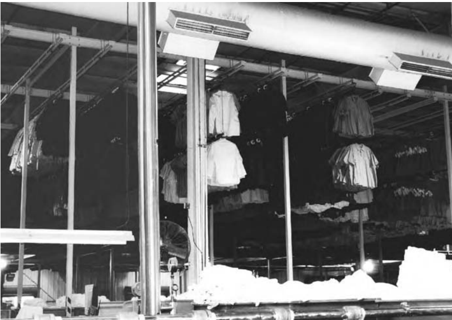
Figure 15-20 The finished uniforms are transported on a conveyor system far above the plant floor, saving valuable floor space. (Photograph courtesy of Mission Industries, Las Vegas.)
