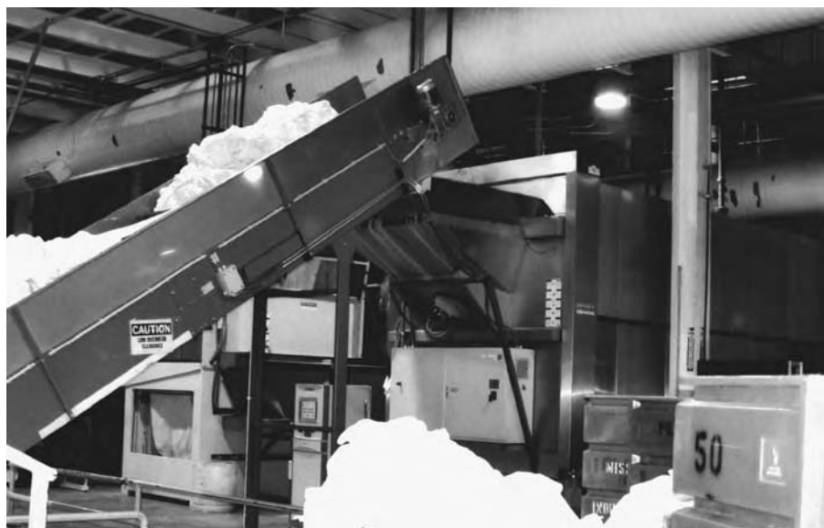
Figure 15-4 The sorted laundry goes up a conveyor into a tunnel washer . These machines can wash up to 3400 pounds of soiled laundry per hour. There are seven of these tunnel washers at this plant. (Photograph courtesy of Mission Industries, Las Vegas.)
