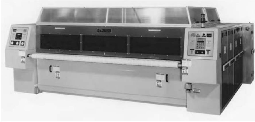
Figure 15-33 The Century Deep Chest All Roll Drive Flatwork Ironer is microprocessor controlled. Because the same control system is used in all aspects of Chicago Dryer's finishing systems, operators need to learn only one system to control the entire finishing area. (Photo courtesy of Chicago Dryer Company.)
