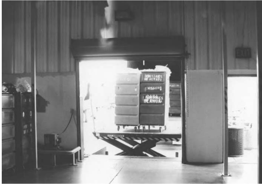
Figure 15-22 Trucks are loaded for return trips to the hotels. The hotels expect and need deliveries every day. Note the lift that raises the carts up to the level of the truck. (Photograph courtesy of Mission Industries, Las Vegas.)
