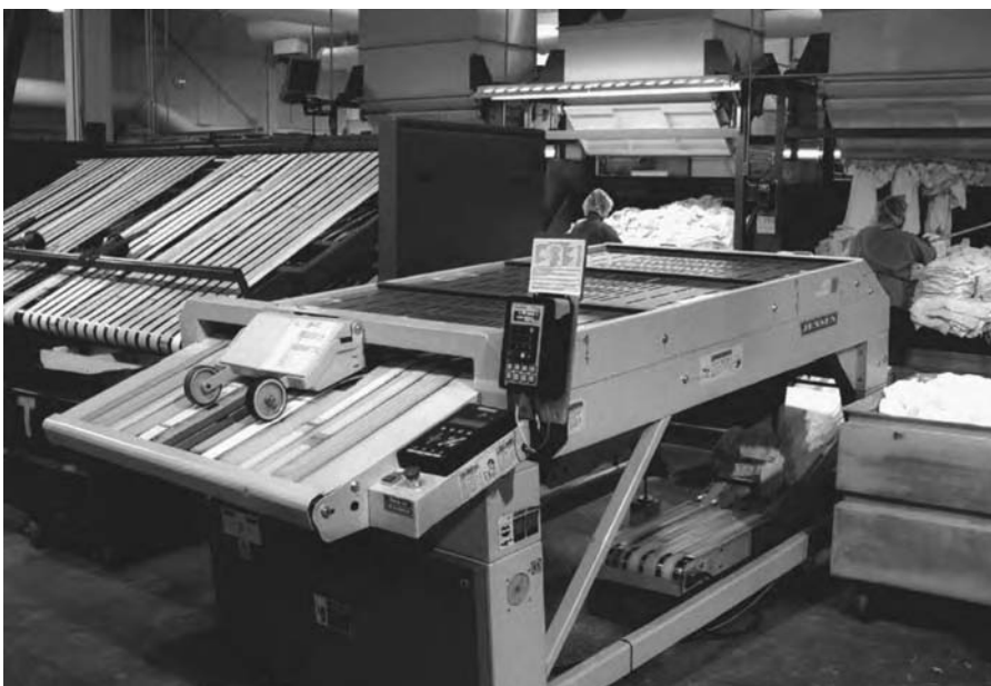
Figure 15-17 Here is a state-of-the-art folder that can fold all sizes of towels with just a push of a button. (Photograph courtesy of Mission Industries, Las Vegas.)
