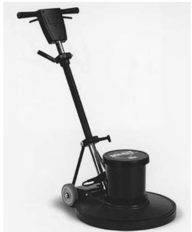
Figure 6-27 The Merit™ Dual Speed Floor Machine has a 175 rpm speed for scrubbing and stripping, and a 300 rpm speed for spray buffing. (Photo courtesy of Windsor Industries, a Castle Rock Company, Englewood, Colorado.)
