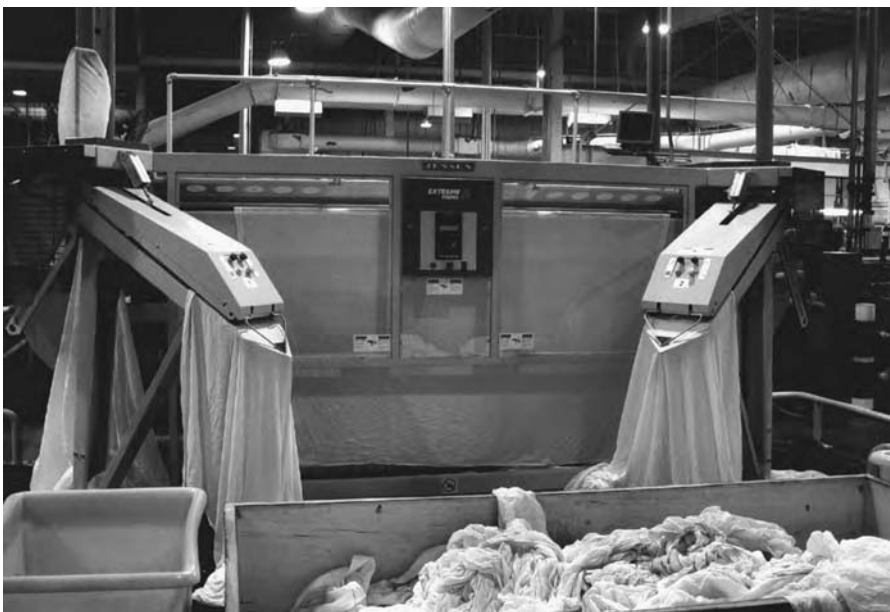
Figure 15-11 Sheets are not dried, but are taken directly from the washers to the flatwork finishers, where they are automatically ironed and folded. A worker only has to find a corner of the sheet and put it into the machine. This flatwork finisher does the rest. (Photograph courtesy of Mission Industries, Las Vegas.)
