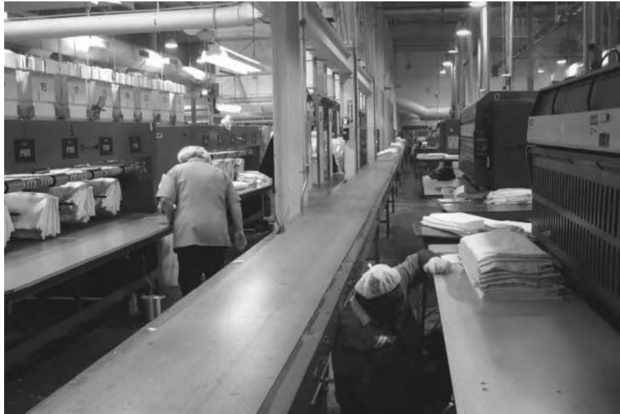
Figure 15-12 The ironed, dried, and folded sheets come out the other side, where workers bundle and place the sheets into carts for transport. (Photograph courtesy of Mission Industries, Las Vegas.)
