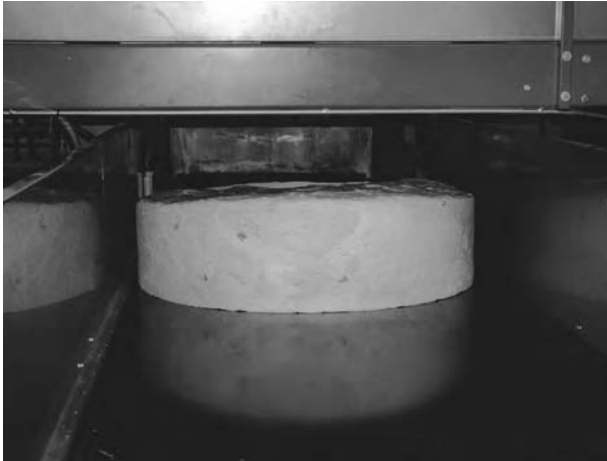
Figure 15-5 After washing, the laundry is pressed to extract water from the fabric. The washer dispenses the clean laundry in the form of 110-pound cakes . The largest tunnel washer produces a 220-pound cake. (Photograph courtesy of Mission Industries, Las Vegas.)
