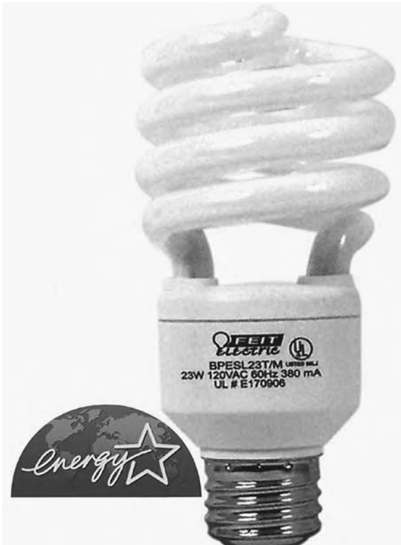
Figure 4-7 A “twist” CFL from Feit Electric. This new design will fit into almost any standard fixture designed for an incandescent lamp. However, these lamps consume only one-fourth the wattage that a standard incandescent would consume. Average rated life is 10,000 hours, as compared with less than 1,000 in an incandescent. (Photo courtesy of Feit Electric, Inc. Pico Rivera, California.)
