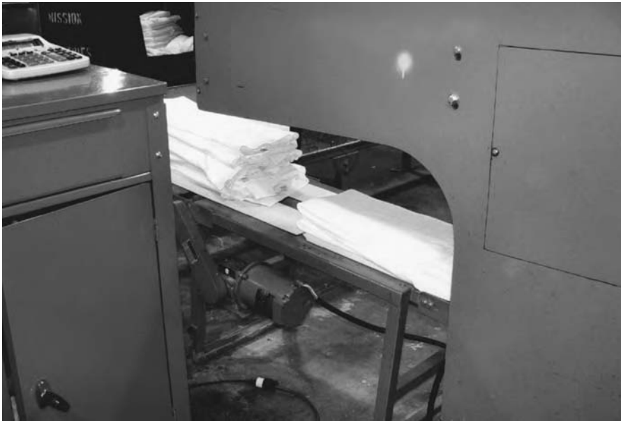
Figure 15-9 The towel is dispensed and automatically stacked on the other side. (Photograph courtesy of Mission Industries, Las Vegas.)
