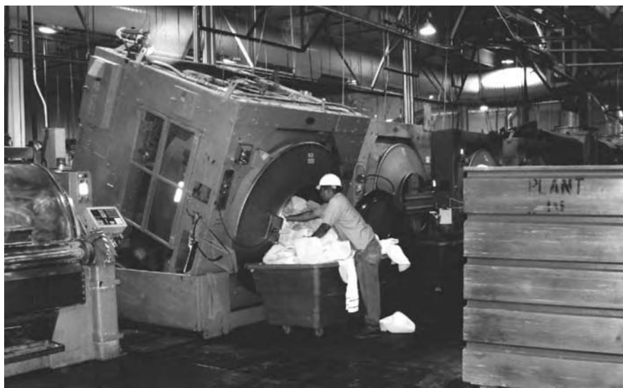
Figure 15-14 Here one of the mid-sized washers is being emptied. Note how the washer tips to aid the worker in emptying the machine. (Photograph courtesy of Mission Industries, Las Vegas.)
