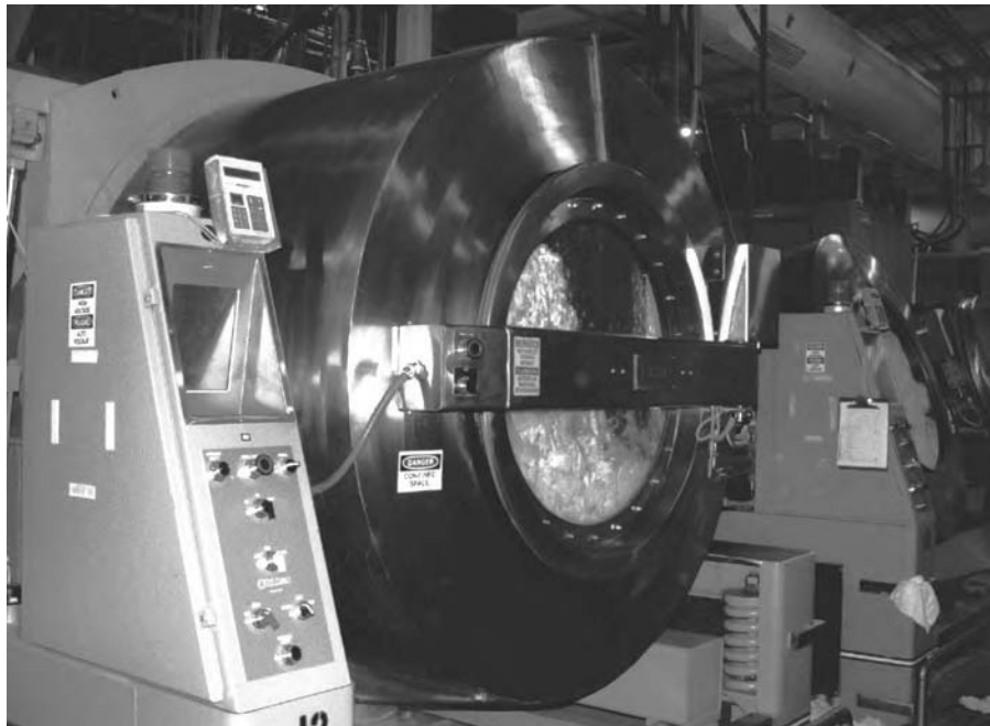
Figure 15-13 In addition to the tunnel washers, the plant has smaller units for uniforms and smaller jobs. The plant has six 125-pound washer-extractors, six 450-pound washer-extractors, and five 900-pound washers with three separate 400-pound centrifugal extractors. (Photograph courtesy of Mission Industries, Las Vegas.)
