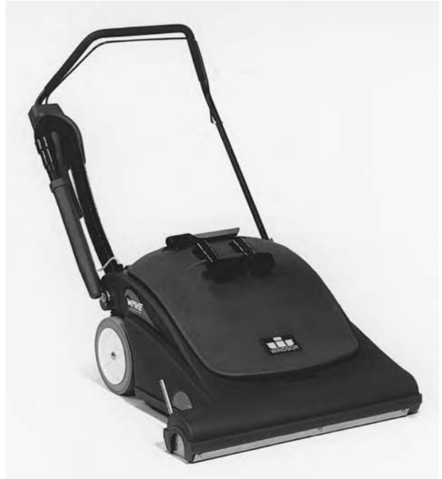
Figure 6-23 The CRI-certified Wave® vacuum has an on-board wand and accessories, two 802-watt motors, a four-stage filtration system, and a 28-inch brush. (Photo courtesy of Windsor Industries, a Castle Rock Company, Englewood, Colorado.)
