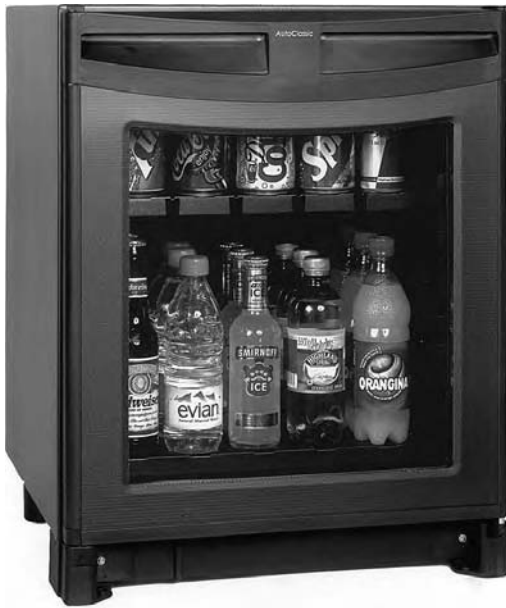
Figure 4-9 This Dometic® auto classic™ refreshment center with see-through glass comes with an infrared sensing system that records each item removed that is not replaced within a preset time period. Its absorption cooling system is superquiet and has no moving parts to wear out. It can link to the front desk through existing television cables.
